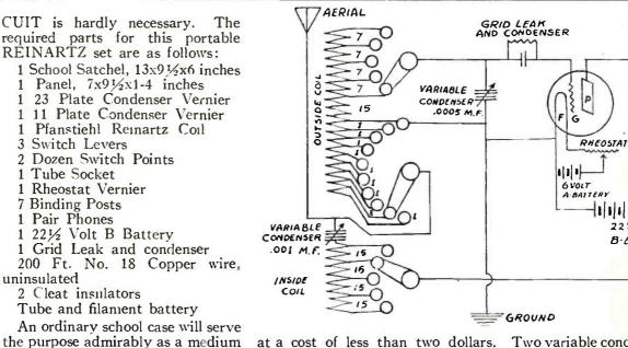
at a cost of less than two dollars. The panel is of bakelite or of other dielectric,  $9\frac{1}{2}$  inches high,  $7\frac{1}{2}$  inches wide and 1-4 inch thick. As all the apparatus is to be mounted on this small panel, care should be taken in the drilling, as space is the most valuable item on the set.
