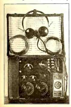
cell is placed in the compartment just to the right of the panel as is the small block 22  $\frac{1}{2}$  volt B Battery.
