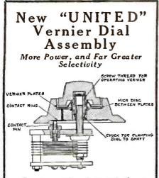
Large capacity, due to the large area of the mica-insulated copper vernier plates.
